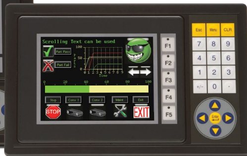
C-more 6" Color Micro-Graphic Panel Installed in a 20-button Landscape Keypad Bezel EA-MG6-BZ2
