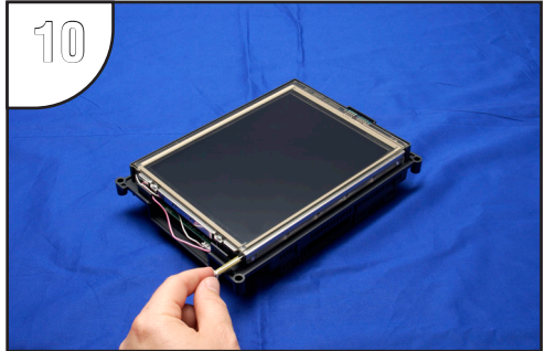
Plug each backlight bulb's power cable connector back into its respective circuit board connector.
