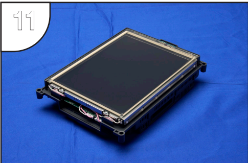
Gently position each backlight bulb's wires back into the wire guides. Position any excess wire length in between the printed circuit board and the LCD to prevent it from becoming pinched between the housing and bezel.
