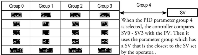
Having PID parameter groups automatically selected for different input ranges allows the system to be more finely tuned or to react differently during the PID or ramp/soak controlled process.
