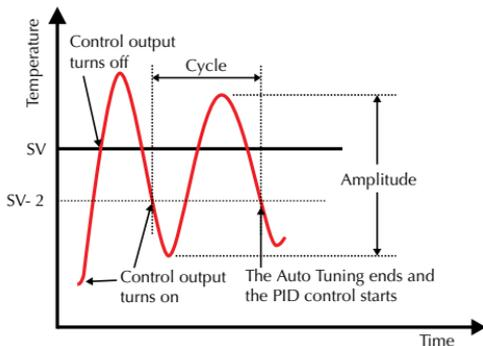
Once the Auto Tuning process is completed, the SOLO controller calculates the above PID parameters for the currently selected group (**Pcd0** - **Pcd3**) and starts the PID control with the new parameter values immediately.
