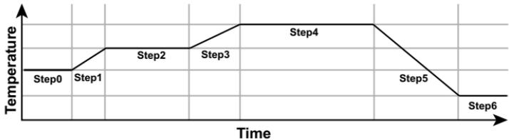
You can select which Ramp / Soak pattern the SOLO controller will execute first. The Ramp / Soak patterns can be executed in series, so the Ramp / Soak control can execute up to 64 steps (8 steps x 8 patterns). You can select which Ramp / Soak pattern will execute next or the controller stops after executing the current pattern. The SOLO controller can execute the same Ramp / Soak pattern up to 200 times before it stops or moves to the next Ramp / Soak pattern.
