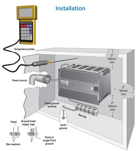
Note: There is a minimum of 2" (50mm) clearance required between the panel door or any devices mounted in the panel door and the nearest DL105 component.
